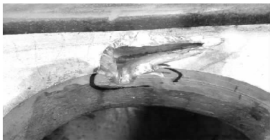
图 6 铸件方盘上部气孔 Fig.6 Gas holes in the square disc of the base
